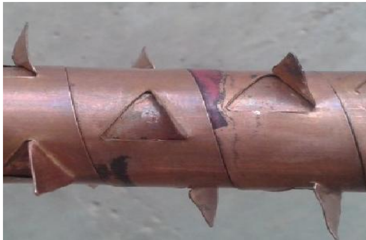
Figure 1: Triangular stripped and Conical type Inserts [6,7]
